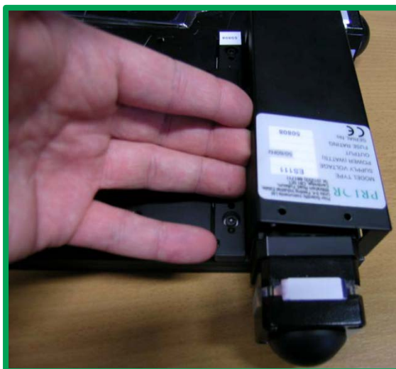
Fig. B: Removal of Y axis drive cover
