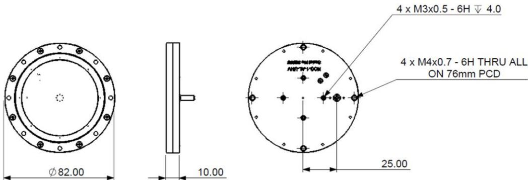
Typically good to  $10^{-10}$  Torr and can be baked out at up to 180°C for two days.
