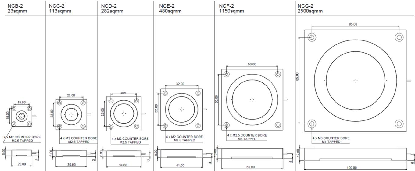
Typically good to  $10^{-10}$  Torr and can be baked out at up to 180°C for two days. Other shapes can be produced on request.
