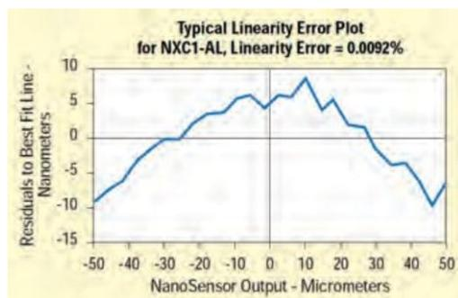
The graph shows the linearity error of a NXC1-AL sensor, in this example it is <0.01%. This is achieved without electronic compensation. Below 0.1%, linearity error is dominated by the parallelism of the mounting surfaces. For the highest linearity choose a large gap sensor and measure over a small part of the full range. For example using NXC1-L sensor over 100um of the 500um calibrated range will give <0.005% linearity.
