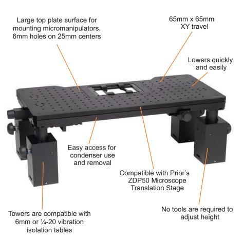
Prior Scientific's patent pending Manual XY Stage ZDeck Quick Adjust Platform enables users to manually adjust the sample XY position with zero electrical noise via X and Y axis knobs. Additionally, the manual XY Stage ZDeck provides users with an ultra stable platform with the flexibility to quickly adjust height for different requirements.
