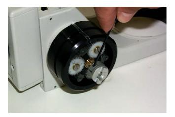
6) Remove the focus motor from the focus adapter by loosening the single set screw. Place the focus adapter over the focus sleeve and tighten the three set screws with the 2mm hex key. Slide the motor in rotate it slowly to make sure that the two mating parts of the coupler interlock. Lock in the motor by tightening the motor lock screw.
