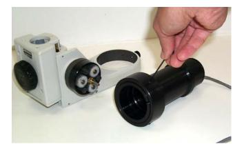
4) Place the focus sleeve onto the focus block and make sure that it is pushed all of the way into the focus block.
