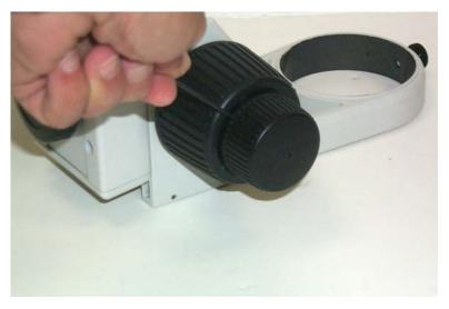
2) Remove the coarse knobs with the Philips screwdriver.
