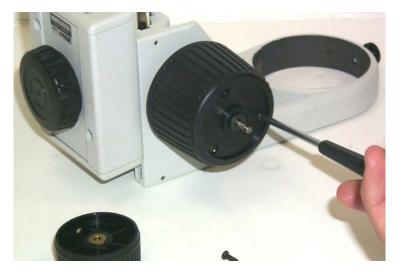
3) Remove the focus sleeve from the focus adapter by loosening the three set screws with the 2mm hex key.
