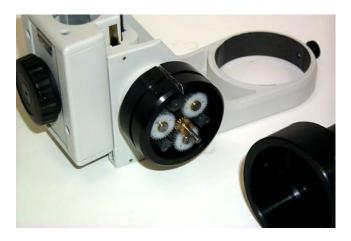
5) Place the silver coupler onto the focus shaft making sure that it does not extend beyond the hole in the coupler. This coupler is either loose in the bag with the focus motor or it is loosely attached to the focus motor shaft via a black anti-backlash coupling. Note that the other coupler attached to the focus motor shaft should not be moved. Tighten the coupler onto the shaft using the 2mm hex key.
