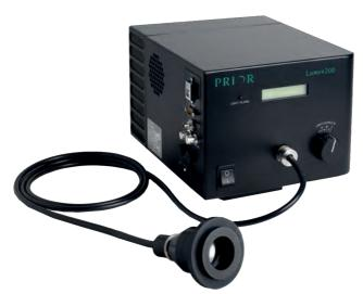
• The Lumen 200Pro has a number of features that further enhance the fluorescence illumination provided by the Lumen 200. The Lumen 200Pro has a mechanical filter wheel, accepting up to 6 filters allowing changes of wavelength within 55 ms, and automatic shutters which can cut off light within 20ms and is controllable via the ProScan III allowing it to be easily integrated into the overall microscopy system.
