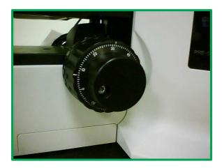
2) Remove the outer fine focus knob as shown below.
