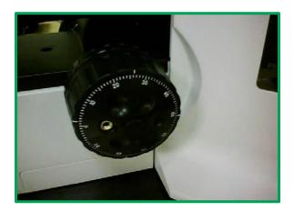
3) Attach the large plastic circular adapter with shaft extension to the inner fine focus knob using the original socket screw, and tighten securely. Attach the inner hub and black anti backlash coupler to the shaft extension as shown below. The outer hub will attach to the actual focus motor shaft and mates with the anti backlash coupler as shown below.
