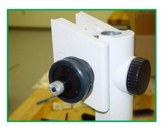
3) Slide the split ring sleeve over the coarse knob. The chamfered end of the sleeve should be outward from the body of the microscope.
