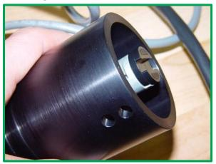
6) Slide the focus motor into the bell housing. Whilst applying gentle pressure inward on the motor tighten the thumb screw. The motor may have to be rotated to set the coupling correctly.
