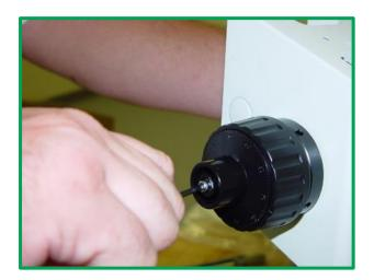
2) Attach hub to assembly using M3 x 25 socket screw and washer divided with focus motor assembly. Take care to make sure the hub and fine focus knob are concentric.
