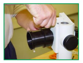
5) Mount the 5 mm hub and black anti-backlash coupler to the end of the focus motor. The hub will tighten to the motor shaft via the screw site on its side.
