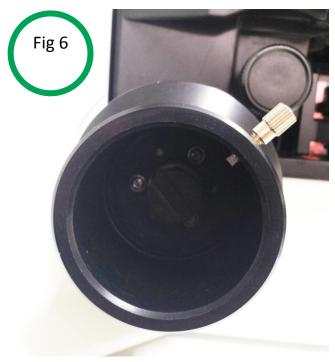
For **NIKON MICROSCOPES**, the procedure is similar; however there is no need for the 'D' adapter. Mount the Nikon (C) coupler (with a different diameter than the (C) coupler for Olympus microscopes to accommodate the Nikon shaft) ensuring the Nikon fine focus shaft goes through it. Proceed with the rest of the installation as outlined above .
