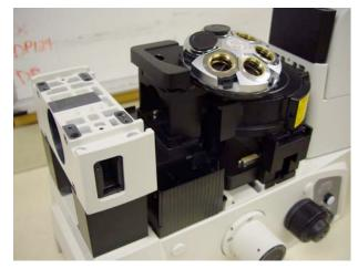
16. Install the front stage riser as shown using the (2) M5 x 60 cap head screws and washers provided. Attach the illumination pillar and epi-fluorescence arm to complete the assembly. Finally, the filter wheel cable must be fitted with the provided hood for right angle exit. The hood should be fitted to the female end of the cable such that the cable exits the wheel toward the rear of the microscope.
