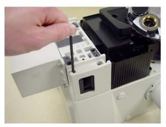
8. Remove the nosepiece and filter turret.
