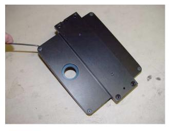
6. Attach turret supports to the base as shown. Note the proper orientation of the supports on the following page.
