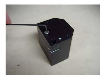
15. Place the pillar riser on top of the riser blocks as shown and secure using the (4) M5 cap head screws provided with the microscope.
