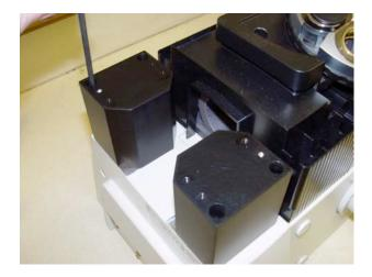
14. Insert screw plate into the slot on each of the riser blocks as shown and fasten using the M4 x 14 countersunk screw provided (the plate is symmetric).
