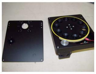
4. Remove the standoffs from either side of the connector and replace them with the provided posts.
