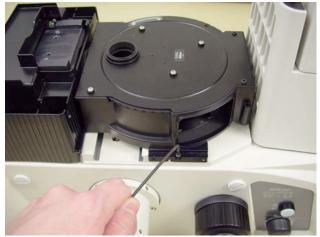
9. Install nosepiece block using (2) M5 x 16 cap head screws and washers provided.
