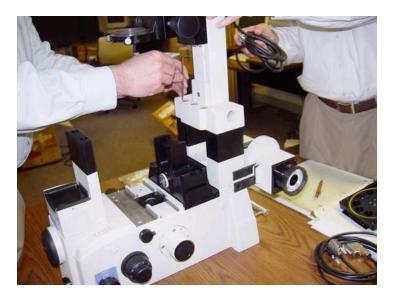
7. Install the Filter Wheel/Turret Block assembly into the original position of the filter turret, using the two M3 x 12 SHCS's provided. Place the light tube over the light path and install the right angled cable.
