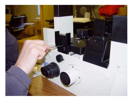
8. Install stage and filter turret. The complete assembly will look as shown below.
