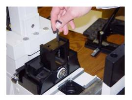
4. Remove Epi-fluorescence attachment and install Epi-fluorescence dovetail riser using the existing set screw as shown below. Re-install Epi-fluorescence attachment using set screw provided in Epi-fluorescence dovetail riser. This must be done before installing the illumination pillar blocks.
