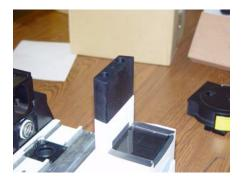
3. Install Nosepiece block using two M5 x 20 SHCS provided as shown below.
