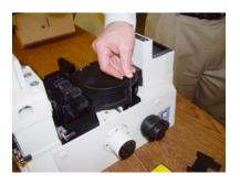
2. Install front stage Riser using two M5 x 60 SHCS provided
