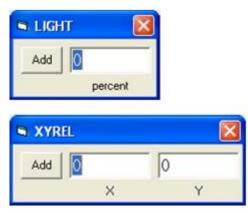
e.g., Type in the % of light you would like the lumen attenuator to allow through.
