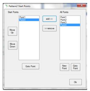
Every time the pattern is run it will start at the start point, if no start point is set the pattern will run from the current position.
