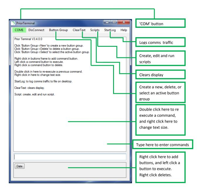
It is important to select the correct COM Port to allow the system to function. This is done by clicking 'Com', which also allows the baud rate to be changed. The default setting of the controllers is 9600; however some software can change this. Once Prior Terminal is open, to list what hardware is connected type '?'. From the product manual you should see the correct response this should generate. For example, from the ProScan III one might get the response:
