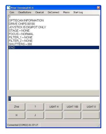
An example of the ? command. This responds back the the information about the peripherals connected to the controller.
