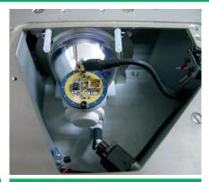
Lift springs and secure lamp in place.
