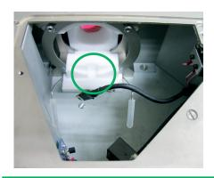
The bulb slots in with the wire into the groove (circled). Connect rear power connector
