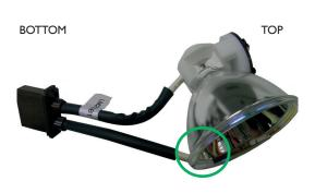
Remove the lamp; orientate as shown. Note wire (circled).
