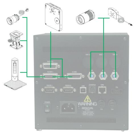
Note that "FILTER I" supports BOTH filter wheels AND focussing-mechanisms
