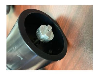
9. Place the other half of silver coupler & black plastic part (not pictured) onto the microscope fine focus shaft and tighten set screw to hold in place.
