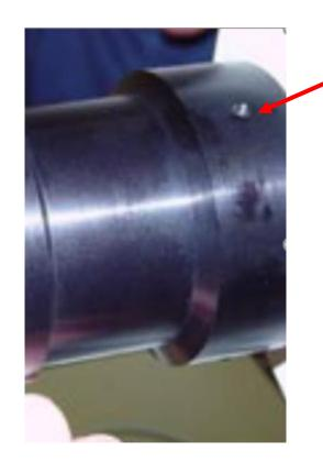
11. Tighten the three set screws in the bell housing to secure the housing to the fixed collar.
