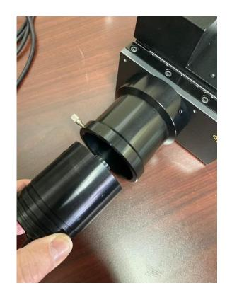
13. Tighten the thumbscrew of the bell housing to hold the motor securely in place. Installation should now be complete.
