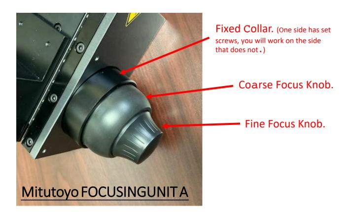
1. Pull off the fine focus knob. It is only held in place by friction.
