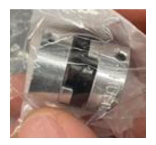
8. Place the silver coupler on the motor shaft and tighten the set screw(s). There is a hole in the motor housing to access the screw.
