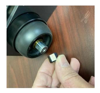
3. Loosen the set screw (not visible in photo) that holds the bushing to the fine focus shaft and slide the bushing off the shaft. It will not be reused.
