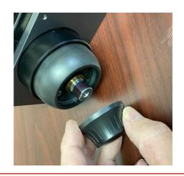
**NOTE:** With fine focus knob removed, if the inside shaft looks as shown, with two small hex nuts at the end of the shaft, stop and push the fine focus knob back into place. You must install the motor onto the other side of the focus block.
