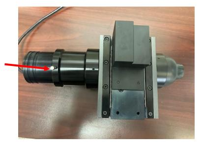
Connect motor to controller and verify smooth operation of the fine focus.
