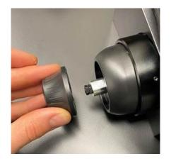
2. There is a thin sheet metal spring sleeve that holds the fine focus knob in place. It may stay with the knob when removed or still be on the aluminum bushing. Remove it from the bushing.
