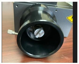
10. Slide the motor bell housing onto the focus block. It should slide all the way onto the fixed collar and rest against the focus block housing.
