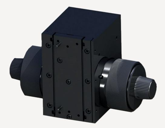
The FB201 from Prior Scientific is a manual focus block, ideal for OEM applications requiring manual, fine focus adjustments. Rack and pinion mount allows smooth, precise focussing over 29 mm of travel. A large coarse focus mechanism incorporates a slip clutch and focus adjustment. Fine focus adjustment control is graduated in two micron divisions throughout the fine focus range. The focus block can be easily adapted to various mounting configurations.
