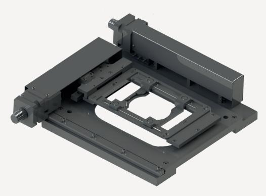
Economical yet precise, the ES107 motorised stage is designed to integrate with the OptiScan control system from Prior Scientific and fits with inverted microscopes. The ES107 offers excellent control over the XY axes for a reduced outlay compared with other motorised stages on the market; ideal for the user who does not require sub micrometre repeatability but nevertheless needs a reliable and accurate stage for routine and repetitive imaging applications.
