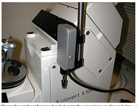
2) Clamp the probe reference bracket onto the nosepiece as shown below, with the glass contact plate facing upwards. Adjust the probe clamp and rob as required to ensure that the probe maintains contact with the glass contact plate over the required range of focus.
