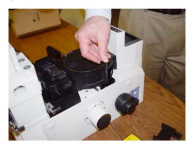
2) Install front stage riser using M5 x 60 socket head cap screws.
