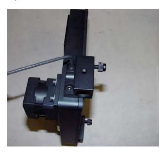
2. Remove the adapter mounting plate
