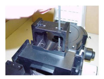
11. Install the filter wheel assembly as shown using the M3 x 10 cap head screws provided. Place the light tube on the aperture of the wheel.
