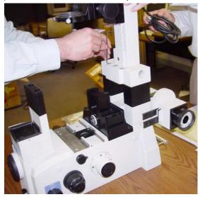
7) Install the filter wheel/turret block assembly into the original position of the filter
