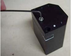
16. Place the pillar riser on top of the riser blocks as shown and secure using the M5  $\times$  60 cap head screws provided with the microscope.
