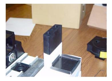
3) Install the nosepiece block using M5 x 20 socket head cap screws as shown below.
