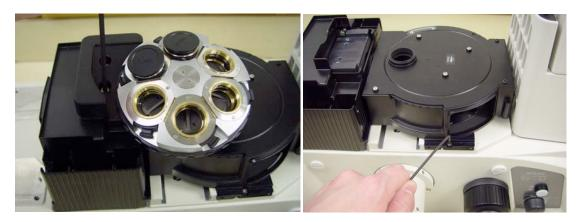
10. Install nosepiece block using the M5 x 16 cap head screws and washers provided.
