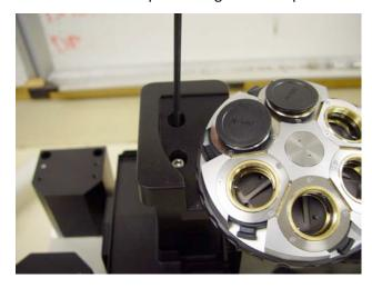
14. Drop the M5 x 50 cap head screws provided through the access holes in each of the pillar riser blocks. Position the blocks on the microscope base as shown and tighten the screws. #
