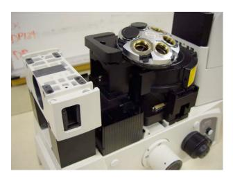
17. Install the front stage riser as shown using the M5 cap head screws and washers provided. Attach the illumination pillar and epi-fluorescence arm to complete the assembly. Finally the filter wheel cable must be fitted with the provided hood for a right angled exit. The hood should be fitted to the female end of the cable such that the cable exits the wheel towards the rear of the microscope.
