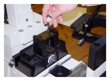
4) Remove epi-fluorescence attachment and install the epi-fluorescence dovetail riser using the existing screw set. Re install the epi-fluorescence attachment using the set screw provided in the epi-fluorescence dovetail riser. This must be done before installing the illumination pillar blocks.
