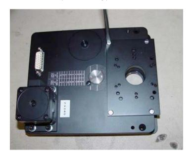
3. Remove the cover plate to expose the inside of the wheel. Set the screws aside – they will be used later.
