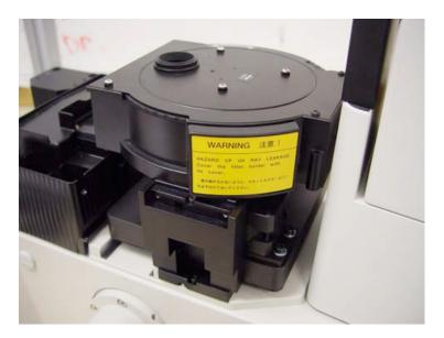
13. Install the nosepiece using the M5 captive fasters provided with the microscope
