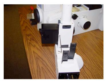
5) Install two pillar blocks to raise the illumination pillar using the four M5 x 60 socket headed cap screws.
