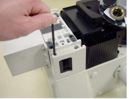
9. Remove the nosepiece and the filter turret.
