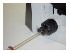
3) Thread the shaft extender onto the fine focus shaft and tighten firmly with your fingers.
