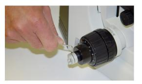
6) Remove the existing rubber coupler from the focus motor shaft and replace with the remaining hub, as shown below.
