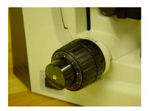
2) Remove slotted brass nut using the flat head screwdriver provided, as shown below. This will expose a threaded shaft. **Do not remove the fine focus knob**.
