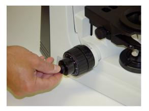
4) Tighten the 3 set screws of the shaft extender into the fine focus knob, ¼ turn at a time as shown below. Tightening the set screws ¼ turn at a time will ensure that the shaft extender stays aligned with the fine focus shaft. You can determine fi the shaft extender is off axis by looking down from above and rotating the fine focus knob. The shaft extender should spin true and not wobble.
