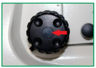
3) Remove the holding screw found behind the cap using the M2.5 HEX wrench provided with the kit.
