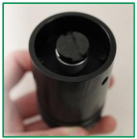
7) Place the focus sleeve provided with the motor in the course focus knob on the left hand side of the microscope.
