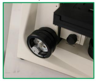
8) Attach the bell housing to the focus sleeve and course knob by sliding the housing over the focus sleeve. At this point, do not attach the three set screws as you may have to slide back the housing during step 9 to make the attachment process easier.
