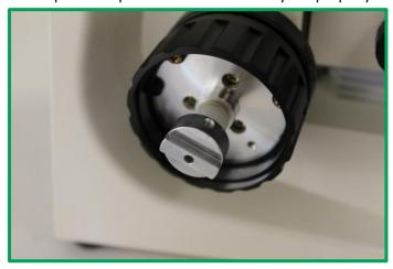
6) Remove the friction pad from the focus motor using a Philips head screw driver and attach the other side of the coupler to the shaft using the 1.5 mm HEX wrench provided with the kit. There are two set screws that will need to be tightened in order to ensure that the coupler is installed securely. Once the coupler is installed, attach the black torque disk to this half of the coupler.
