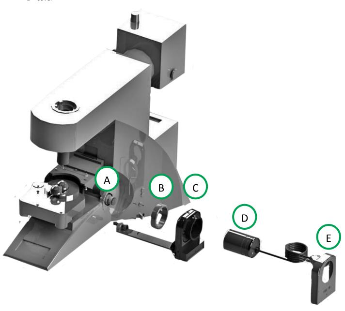
Remove the right hand side focus knob of the Leica DM4000, exposing the fine focus spindle.
