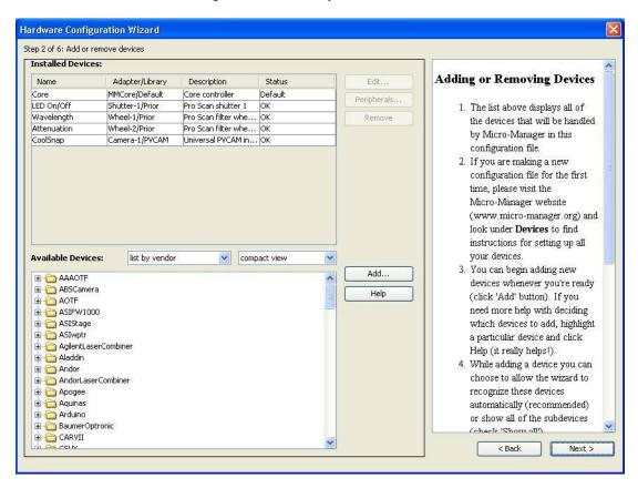
Remember at the point to add any other Prior equipment (eg stages, shutters, filter wheels) and any other external hardware (eg microscopes, cameras etc), before moving onto the next step. In this example a CoolSnap camera was also added.
