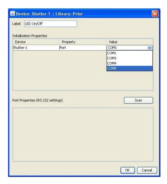
Change the label to identify the shutter as eg "LED On/Off".
