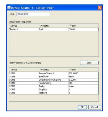
Make sure the correct values are set for the Baud rate etc (see above).
