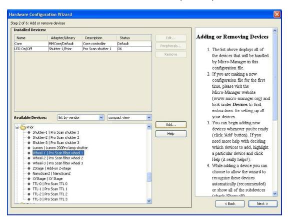
Select the following devices 'Wheel-1 | Pro Scan filter wheel 1' and click 'Add'. Set up the correct COM ports as with the Shutter.
