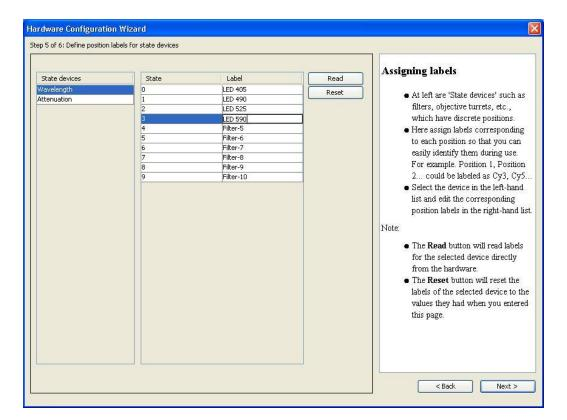
The properties of the filter wheels can be set in "*Define Position Labels for State Devices*" Under Wavelength type in the wavelength properties for each of your LEDS. Note 0 is Filter wheel position 1.
