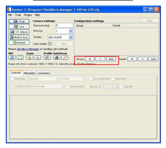
To get quick access to changing wavelength and attenuation of the LEDS it is best to set up Groups. Click on the + sign to add a new Group.
