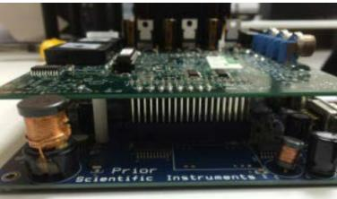
Reconnect the connectors and secure the board in the ProScan II case
