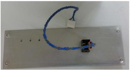
The back panel, with the associated main board, can then be simply slide out of the casing by undoing the four screws on the back panel.
