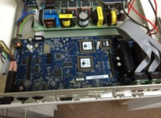
Fit the filter wheel and shutter board to the main board
