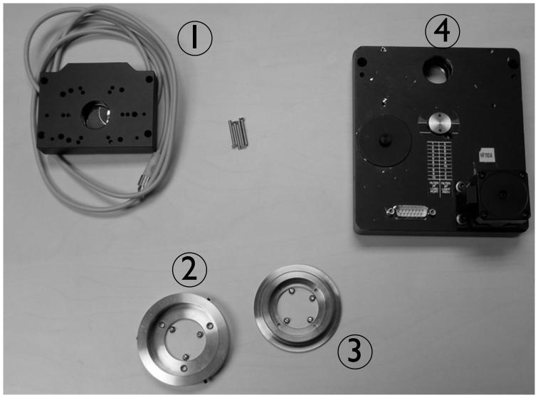
By the end, the microscope should be attached to the shutter via the microscope adapter. The silver side of the shutter should face towards the light source. The shutter is attached to the filter wheel, which in turn is attached to the light source via the light source adapter.
