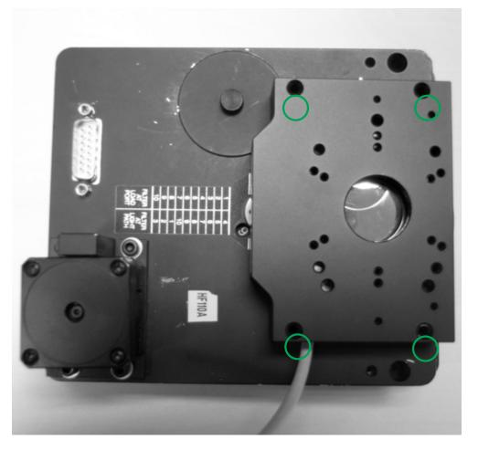
Line up the other adapter and screw that in. The shutter is now installed onto the filter wheel.
