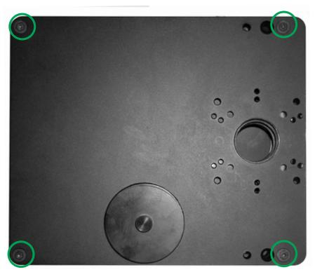
Remove the backplate. Teh adapter is placed on the backplate exterior, however the screws must be inserted and screwed in from the opposite side. Once the adapter is securely attached reattach the back plate.
