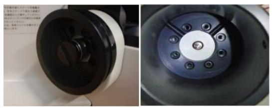
Attach the focus motor sleeve to the mounting flange using the grub screws.
