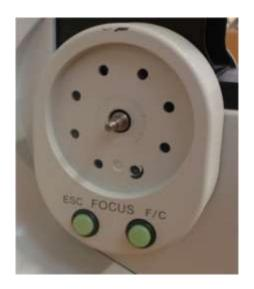
Put Black collar over the microscope spindle and faster with the metal hub grub screw.
