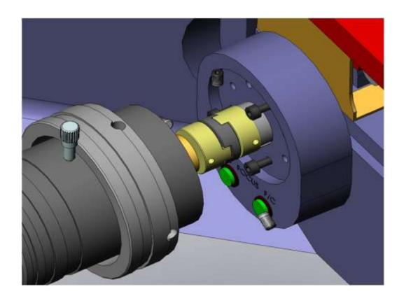
Remove the Left hand focus knob from the Olympus microscope.
