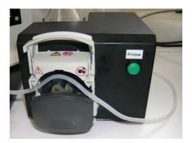
Clamp the tubing in the pump as shown.
