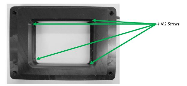
• Secure the Prior sample holder by alternately and evenly tightening the four captive screws (shown above), while making sure that no torque is applied between the outer frame and inner stage.
