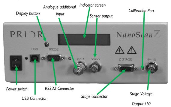
Note: Please ensure you note the position of the Stage and RS232 connections, it is important to connect these correctly.
