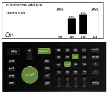
Press and hold a White Mode preset button for 3 seconds. On releasing the button the display will temporarily indicate that the selection has been saved to that specific White Mode preset
