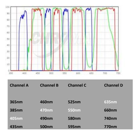
In the above example a DAPI/FITC/TRITC/Cy5 quad filter is excited by 405nm, 470nm, 550nm and 635nm.
