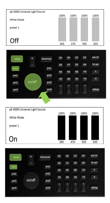
Use master intensity control to vary all intensities in 1% steps. The display indicates the variation from the preset value. If the intensities are set at different values, then the balance between the channels will be maintained. The range of the adjustment is limited to the lowest intensity reaching 0% and the highest intensity reaching 100%.
