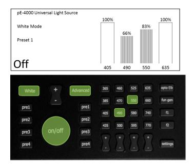
Press 'White' button to change to White mode. The last pre-set button used becomes the selected one. In going from 'Advanced' mode to 'White' mode the on/off status automatically goes to off.
