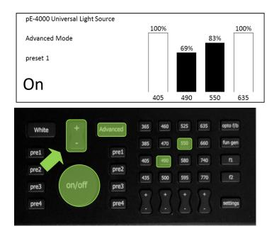
To save wavelength and intensity selection, press and hold for 3 seconds one of the advanced preset buttons. The display will indicate once the selection has been saved to the specific preset button.
