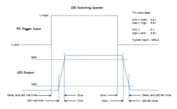
With fast repetitive switching, the pod display will not be able to respond at the same speed and so can get out of synch. If after a train of pulsing, the display on the Pod indicates that the LEDs are on while they are actually off, simply press the on/off button to reset the display correctly.
