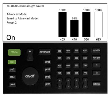
Press the on/off button to switch on the LEDs and operate the pod as per section 8.
