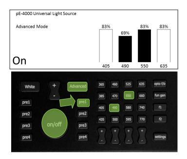
With no wavelength selected, pressing the on/off button will have no effect except the display will indicated that no wavelength is selected.
