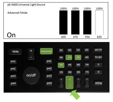
Reduce the intensities of all channels in 1% steps with the use of the master intensity button. The balance between channels will be maintained.
