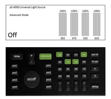
Press alternative wavelength to change channel selection. The intensity of the newly selected wavelength will be the same as it was, the last time it was selected in Advanced Mode.
