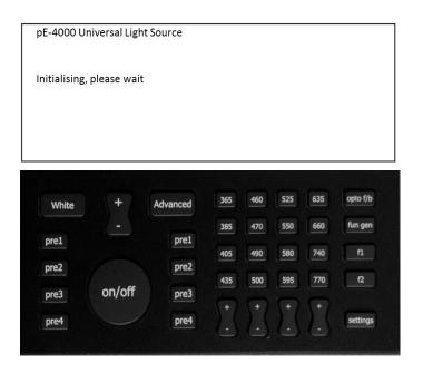
Once initialised, the system defaults to White Mode and to the preset that was last used at previous power down. There will always be one preset active. The buttons which are active are backlit. In White Mode all the advanced buttons are disabled (except for 'Advanced'). The display indicates the wavelength selection and their intensities for the active preset.
