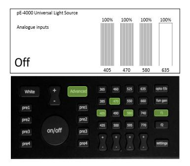
Press the wavelength button corresponding to the wavelength which is required to be under analogue control. The symbol on the screen will change to an icon representing analogue control.
