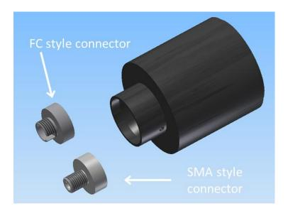
2) To change between SMA and FC, simply release the grub screw on the side of the collar which releases the connector and replace with alternative, ensuring that it is fully inserted before tightening up the grub screw.
