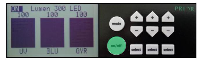
The control pod enables the user to control the intensity of the LEDs that are exciting different stains. This helps to balance the emissions so that one stain does not dominate another. This feature is very useful in multi-band work (see Appendix).
