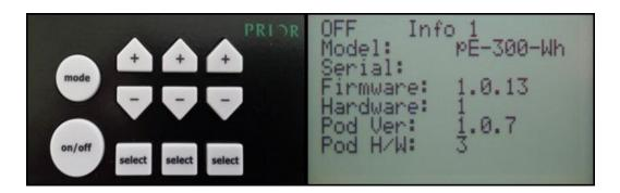
To find out how long the LEDs have been lit, press and hold the 'mode' button for 3 seconds. Once the display settings screen appears , release the 'mode' button and then give two short duration presses to retrieve this information. Wait 10 seconds to return to the main screen or alternatively press and hold the 'mode' button for 3 seconds.
