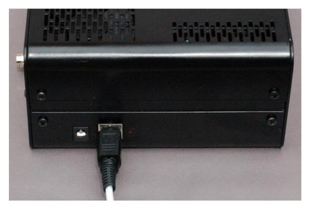
Connect the power connector from the DC power supply. At this stage do not connect the mains power lead to the DC power supply.
