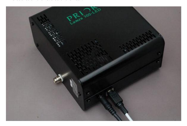
The TTL signal controls the on/off function of the unit. A TTL 'high' will cause the LEDs to be on, independent of the state of the on/off button, however only those bands which have been manually selected on the pod will be switched by the TTL signal. The intensities of the selected bands are manually set on the pod.
