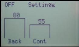
To interrogate the product on its firmware and hardware, press and hold the 'mode' button for 3 seconds. Once the display settings screen appears , release the 'mode' button and then give it a second short duration press. The screen will display the relevant information. To return to the main screen, either press and hold the 'mode' button for three seconds or wait for 10 seconds for the screen to automatically return.
