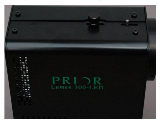
To make the adjustment, set up a typical sample on the microscope that gives an image over the whole field of view. Loosen the thumbscrew and move the post back and forth until you get the brightest and most even illumination possible. Tighten the screw again when finished.
