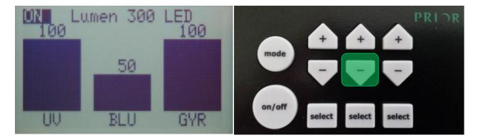
Individual bands can be switched off entirely. This can improve contrast ad cell viability and well as save energy. Switching off UV, in particular, will reduce photo-bleaching and damage of samples. Bands can be switched off by pressing the 'on/off' button and switched on again by pressing the 'on/off' button again.
