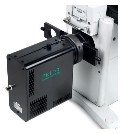
Ensure that there is free airflow around the LED head so that the cooling system is not impaired. A gap of 200mm on either side is sufficient. Ideally the unit should be upright, but it may be set with the cables at the top or at either side.
