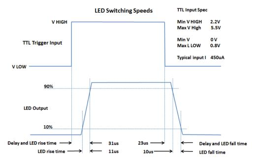
The TTL input circuit has been designed to maximise the switching speed of the LEDs to give the user precise control of the excitation light reaching the sample.
