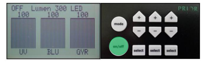
To switch on the LEDs press 'on/off' once. To switch them off again press 'on/off' again.
