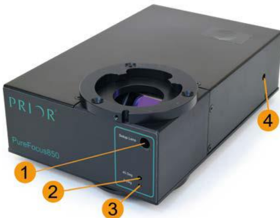
Figure 5: Setup (1), 45 degree (2), 0 degree (3) and blade (4) adjustment screws.
