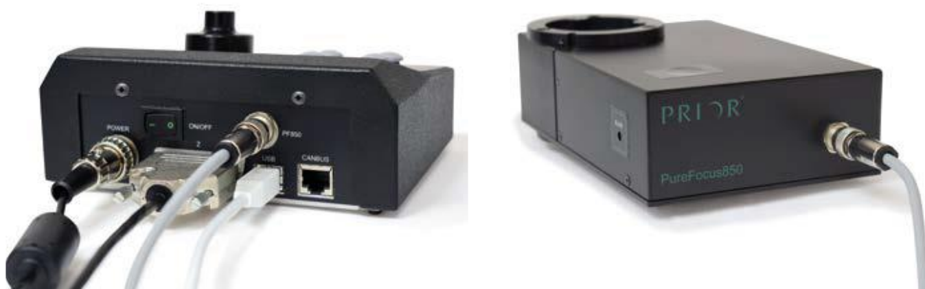
Figure 3: Controller and head connections.
