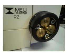
Attach the bell housing to the focus sleeve via the 3 set screws on the OD, making sure to tighten the set screw at roughly a 90 degree angle from the slot in the focus sleeve first.
