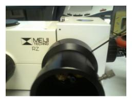
Attach the other hub from the coupling to the focus motor. (this may have been done at the factory)
