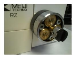
Place the focus adapter sleeve H2531 over the focus gear assembly housing
