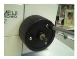
Remove coarse knob exposing the focus gear assembly housing.
