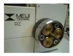
Mount hub to fine focus shaft via set screws.
