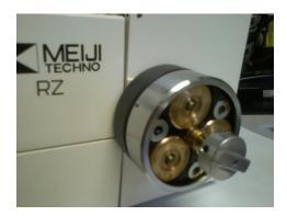
Push black anti-backlash coupling onto hub, making sure to align the OD of both.
