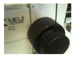
Remove 3 phillips head screws holding coarse focus knob to focus assembly.
