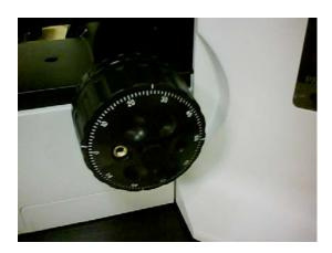
3. Attach large plastic circular adapter with shaft extension to the inner fine focus knob using the original socket screw and tighten securely. Attach the inner hub and black anti-backlash coupler to the shaft extension as shown below. The outer hub will attach to the actual focus motor shaft and mates with the anti-backlash coupler as shown below.
