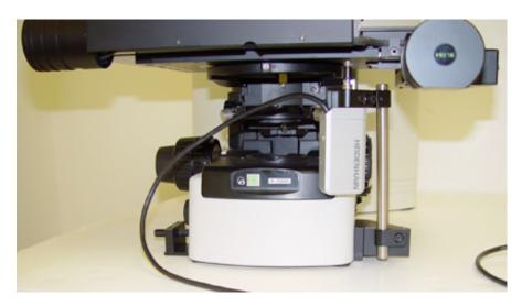
3. Adjust the probe plunger so that it contacts the bottom of the stage making sure that it is clear of any tapped holes on the stage. Adjust the height of the probe so that it maintains contact with the baseplate over the required range of focus.
