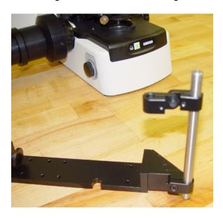
2. Place clamp plate under microscope just behind the microscope mounting feet and tighten clamp with flat head screwdriver as shown below.
