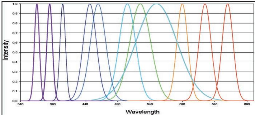
Eleven different LEDs are available. The 11 LEDs above each provide a narrow spectrum of light for specific fluorescent purposes. A white light LED is also available, giving a broad spectrum of light.
