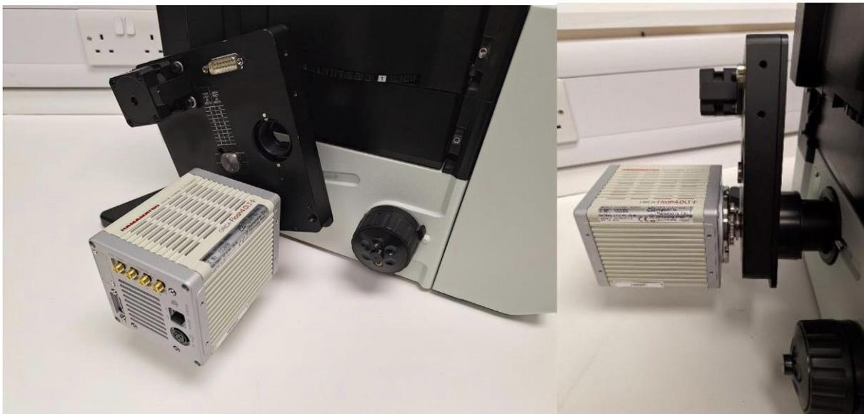
5. When the filter wheel is installed, screw the camera onto the C-mount adapter until you achieve parfocality between your camera and the eyepiece. Once the correct position has been found, rotate the lock ring of the adapter towards the camera to lock the camera in place.
