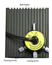
F. Remove the paper and using the 10x objective view a metallurgical specimen. If there is any shadowing in the field of view carefully adjust the bulb focus until it disappears.
