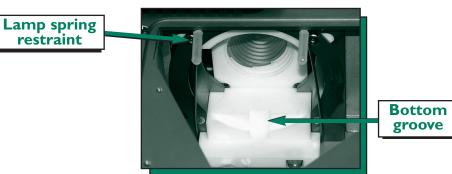
Lift the spring towards the bulb, as you do the bulb will be pushed into the correct position. Click the springs all the way into the lamp spring restraints (see images below).
