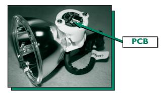
Locate the bottom of the bulb (as indicated in the above photo). Place the wire at the bottom of the bulb into the groove in the bottom of the lamp chamber (as indicated below). Center the bulb in the circular lamp mount.
