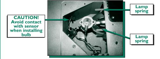
With the bulb now firmly in place, plug the data connector into the PCB.
