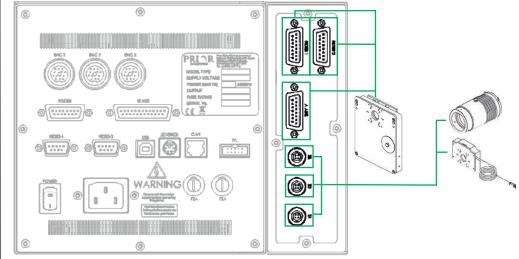
**\_\_\_\_** Encoded connection between ProScan III and encoded Prior device
