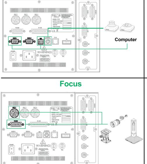
Connection between ProScan III and Prior device
