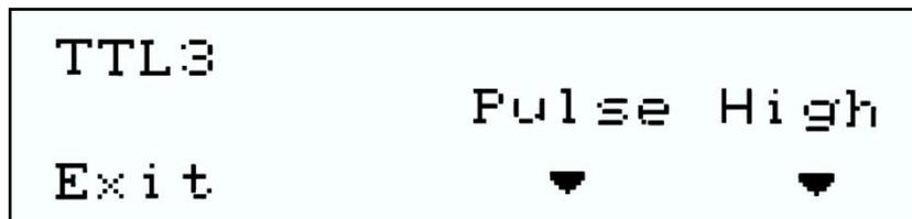
Scroll with the left hand wheel to select which TTL output is required.
