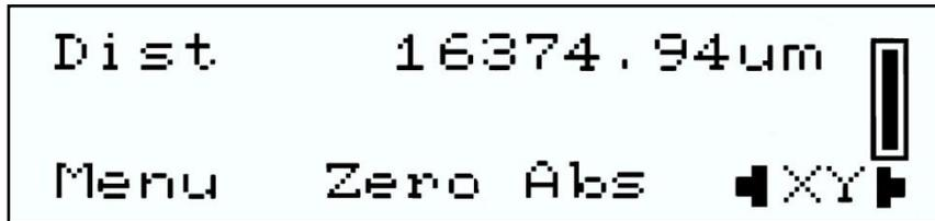
The relative position is replaced by the distance from 0, (0 abs 0, or position when zero button was pressed).
