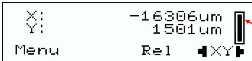
Stage Joystick speed indicator. Pressing button 6 will toggle speed between 25, 50, and 100%.
