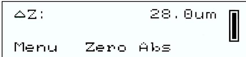
The absolute position is replaced by the relative position.
