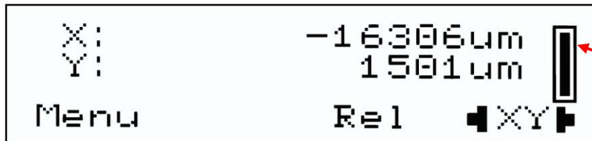
Stage Joystick speed indicator. Pressing button 6 will toggle speed between 25, 50, and 100%.
