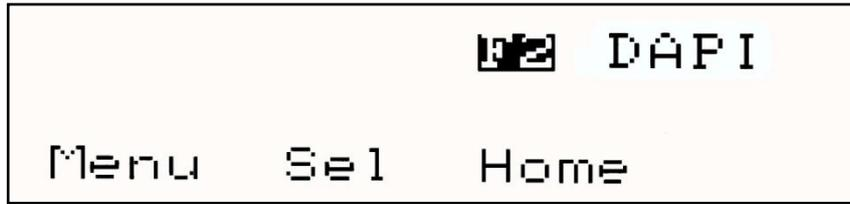
The positions of filter wheels can be named to help you remember which filters set are in which location. These names called “tags” are displayed on the control centre display once they have been set. Each Filter position in each filter wheel can be given a unique name. Use the following ASCII commands sent via RS232 through a terminal or via the VBDemo program supplied free on the Prior Website [www.prior.com](http://www.prior.com).
