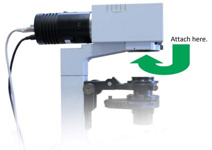
The adapter plate should be attached onto the microscope frame using the 4 small screws provided. The adapter plate attaches to the microscope via the 4 screw sockets circled in green.
