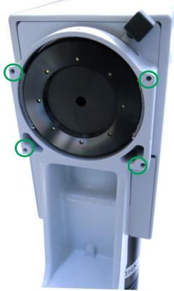
The Shutter is then attached to the adapter plate, using the two longer screws provided. Please note that the screws replace the existing screws inside the shutter unit. Ensure the shutter, adapter plate, and the microscope had are all aligned.
