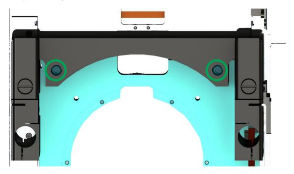
Slightly loosen the leg clamping screws (ringed) to allow the legs to fit into the holes (highlighted green) on the Front Stage bracket.
