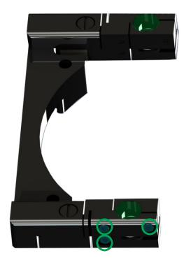
Lower the stage onto the microscope making sure that the legs fit into the corresponding holes in the Front Stage Bracket. DO NOT TIGHTEN THE LEG CLAMPING SCREWS YET.
