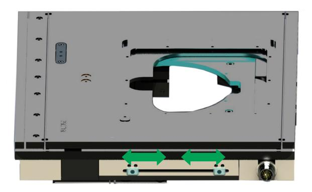
Use an Allen Key to slightly loosen the front or back limit switches and slide the limit along the groove until the desired position has been reached. Once the desired position has been reached tighten the limit switch to prevent it being moved as the stage travels.
