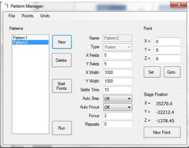
Select the number of X Fields and Y Fields. Select the X width Y width and the (FOV) fields of view, in microns.
