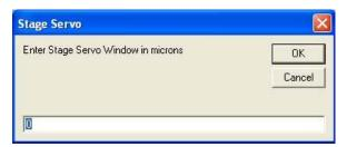
When in servo mode the controller will attempt to keep the focus at a particular position. The servo window is the number of encoder counts the focus can move before the controller will respond and correct the position.
