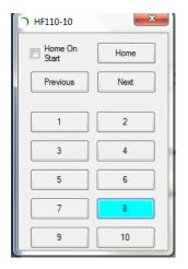
Click 'Next' to move the next filter wheel position. Click 'Previous' to move the previous filter wheel position. Click 'Home' to home the Filter wheel. Check the 'Home on start', to activate the home on startup feature which will automatically home the filter wheel when the ProScan unit is powered on.
