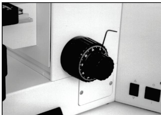
**STEP 2)** Place the spring over the fine focus shaft and place a coupling hub on the shaft whilst holding the opposite focus knob in position, or it may disengage from gears.
