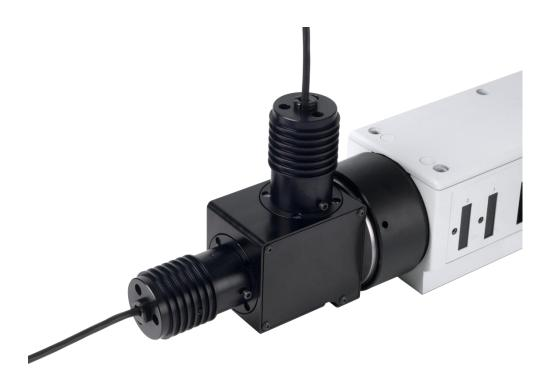
A dichroic mirror will have to be fitted inside the combiner to ensure that both desired wavelengths enter the light path. A dichroic mirror allows wavelengths below a certain value to pass through, whilst reflecting those at a higher wavelength. Therefore, the two Lumen 100 LEDs must be placed correctly, with the higher wavelength LED in such a position that its light will be reflected into the light path. See the diagram below.
