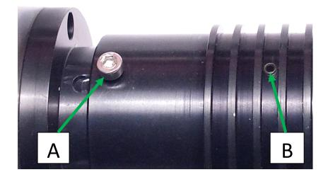
• To centre, first focus the microscope onto a suitable sample, such as an autofluorescent plastic slide (available from Chroma Technology Corp). Use the hex key to undo the centre locking screws (B on the image above), allowing the top half of the LED unit to move freely in a circular motion. Look at the image and check the flatness of illumination. Adjust the position of the LED unit until you achieve a homogenous illumination across the field of view.
