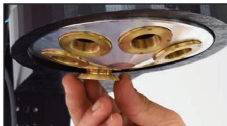
**STEP 2:** Insert the microscope thread adapter.
