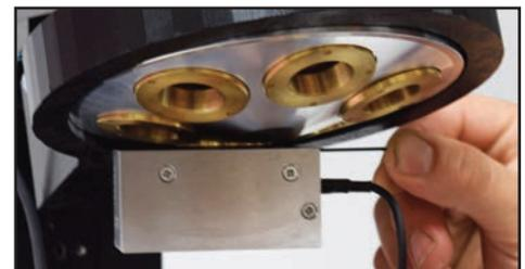
**STEP 3:** Connect the OP400 to the nosepiece. Tighten with the hex key.
