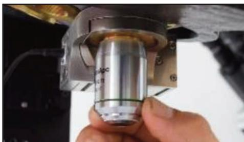
**STEP 4:** Insert the objective lens using the appropriate objective lens adapter. Note no adapter is necessary for M32. Other objectives can be inserted into the nose piece using option parfocal spacers.
