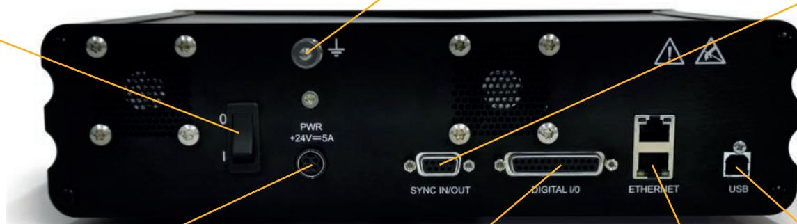
Power Connector 4 pin miniDIN with screen Input +24V dc  $\pm 0.75V$  @ 5A Provides power to the controller electronics. ONLY connect an approved power supply.
